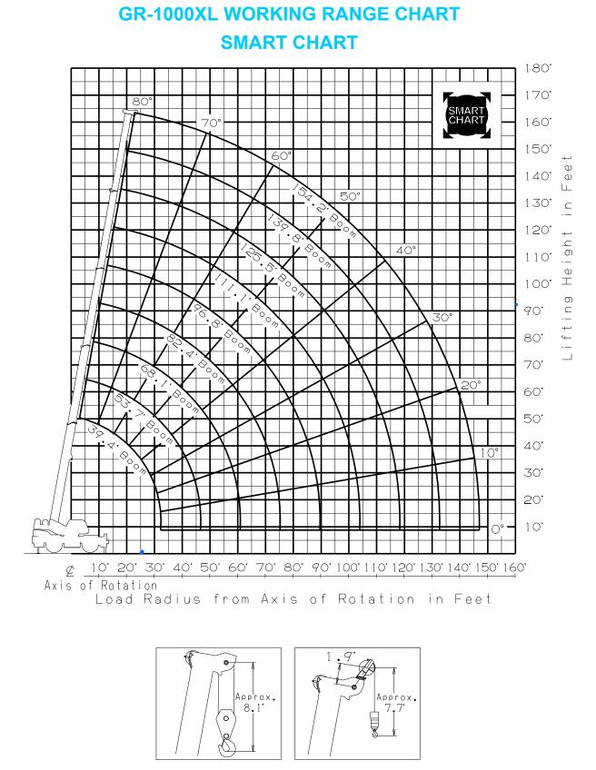
NOTE:1.Boom geometry shown is for unloaded condition and machine standing level on firm supporting surface. Boom deflection and subsequent radius and boom angle change must be accounted for when applying load to hook.
